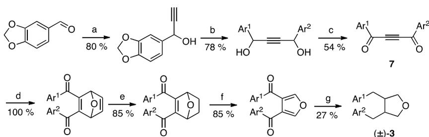
**Reagents and conditions:** (a) ethyne, EtMgBr, THF; (b) Ar<sup>2</sup>CHO, EtMgBr, THF; (c) CrO<sub>3</sub>, acetone; (d) furan, 50 °C; (e) Pd/BaSO<sub>4</sub> (H<sub>2</sub>), EtOAc; (f) 200–250 °C, 0.1 mm; (g) Pd/BaSO<sub>4</sub> (H<sub>2</sub>), AcOH. Ar<sup>1</sup> = 3,4-methylenedioxyphenyl; Ar<sup>2</sup> = 3,4,5-trimethoxyphenyl.
