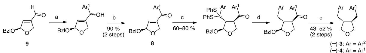
**Reagents and conditions:** (a) Ar<sup>1</sup>MgBr, THF; (b) CrO<sub>3</sub>, CH<sub>2</sub>Cl<sub>2</sub>; (c) (PhS)<sub>2</sub>CHAr, BuLi, THF, -78 °C; (d) Raney-Ni, CH<sub>3</sub>OCH<sub>2</sub>CH<sub>2</sub>OCH<sub>3</sub>, 0 °C; (e) CH<sub>3</sub>COOH, Pd/C, H<sub>2</sub> (1 atm). Ar<sup>1</sup> = 3,4-methylenedioxyphenyl; Ar<sup>2</sup> = 3,4,5-trimethoxyphenyl.
