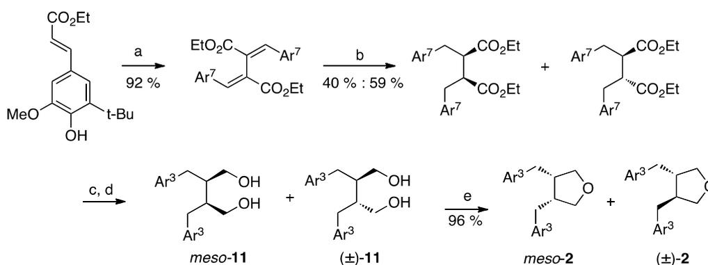
*Reagents and conditions:* (a)  $\text{K}_3[\text{Fe}(\text{CN})_6]$ ,  $\text{KOH}$ ,  $\text{C}_6\text{H}_6/\text{H}_2\text{O}$ , rt, 0.5 h; (b)  $\text{H}_2$ ,  $\text{Pd}/\text{C}$  (10%), rt, 24 h; (c)  $\text{AlCl}_3$ ,  $\text{C}_6\text{H}_6$ , 50 °C, 1 h (79%); (d)  $\text{LiAlH}_4$ ,  $\text{Et}_2\text{O}$ , –15 °C, 2 h (85%); (e)  $\text{HCl}$ ,  $\text{MeOH}$ , reflux, 18 h.  $\text{Ar}^3 = 4$ -hydroxy-3-methoxyphenyl,  $\text{Ar}^7 = 4$ -hydroxy-3-methoxy-5-*tert*-butylphenyl.
