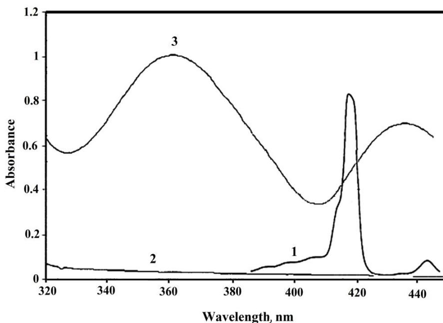
**Figure 2.** Absorption Spectra of: (1) Catalyst 2a; (2) Bromine (3) Catalyst 2a:Br<sub>2</sub> with Molar ratio 0.2:1 in Dichloromethane Solution.
