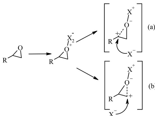
Based on our study on the complexation of porphyrins and other works reported on the different compounds with elemental halogen [23,24,26], it seems that halogenative cleavage of epoxides occurs via trihalide ion,  $X_3^-$  as the nucleophile. In support of this suggestion, the electronic absorption spectra of catalyst (1), iodine (2) and complex formation between iodine and bromine in the presence of 2a as catalyst (3) in dichloromethane solution at 25 °C are shown in Figures 1 and 2.
