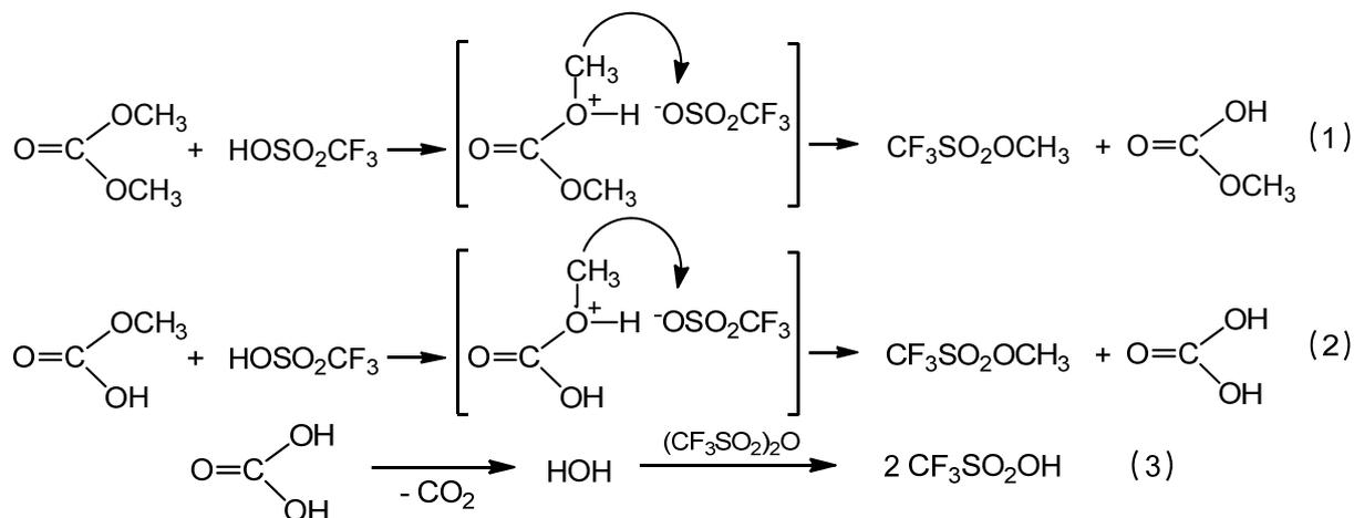
In the first step triflic acid protonates dimethyl carbonate (Equation 1) inducing the methyl cation transfer to the triflate anion resulting in methyl triflate (Equations 1 and 2). Triflic acid is regenerated in the reaction of triflic anhydride with the water which is formed by decomposition of carbonic acid (Scheme 5, Equation 3). According to this mechanism the triflic acid anhydride plays a role as water scavenger.
