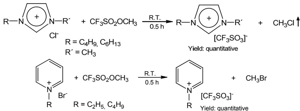
This is a very convenient method to prepare triflate ionic liquids with various substituents R and R'. The reaction progresses very fast at room temperature under solvent free conditions. The gaseous CH<sub>3</sub>Cl or very volatile CH<sub>3</sub>Br are the only side products in this process. Trimethylsilyl triflate is less active in these reactions, but more convenient to handle [42,43]. The side product, trimethylchlorosilane, can be easily utilised.
