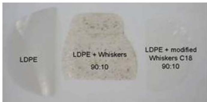
An attempt to use a recently patented concept (Dispersed Nano-Objects Protective Encapsulation - DOPE process) intended to disperse carbon nanotubes in polymeric matrices was reported. Physically cross-linked alginate capsules were successfully formed in the presence of either cellulose whiskers or microfibrillated cellulose [92]. The ensuing capsules have been extruded with a thermoplastic material.
