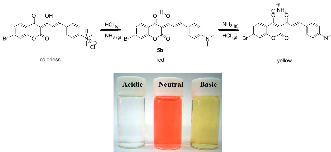
Scheme 3. The acidichromic switch of 5b and the corresponding colors in acidic, neutral and basic conditions.
