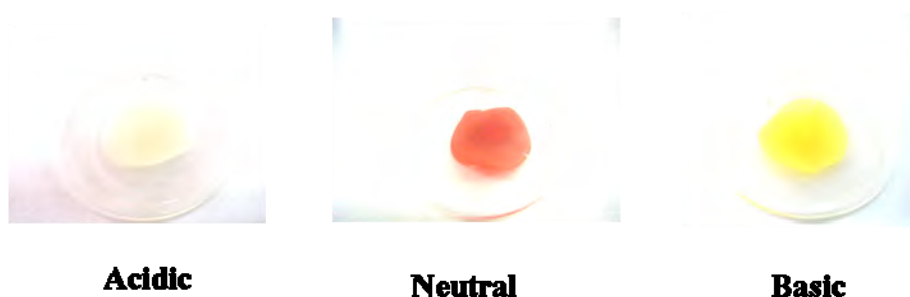
Figure 4. Colors of 5b on PC film under acidic (exposed to \text{HCl}(\text{g}) ), neutral (exposed to \text{NH}_3(\text{g}) ) conditions.
