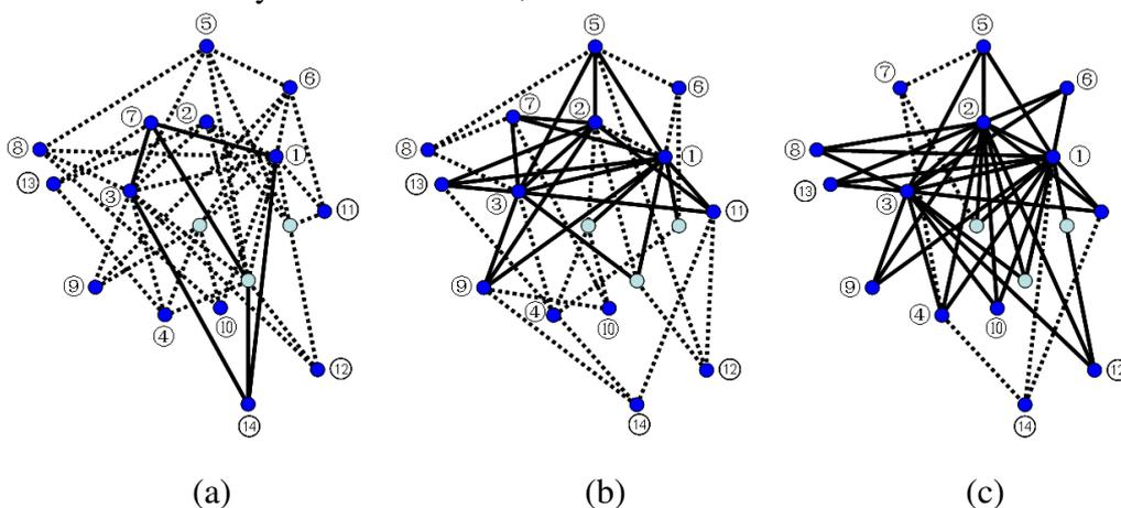
**Figure 1.** The network's evolution process according to different  $d/r$  in  $HUHPM$  model. And the number of nodes is  $N=14$ ,  $m=m_0=3$ . Fig(a) for  $d/r=1/6$ , Fig(b) for  $d/r=1/1$  and Fig(c) for  $d/r=6/1$ .
