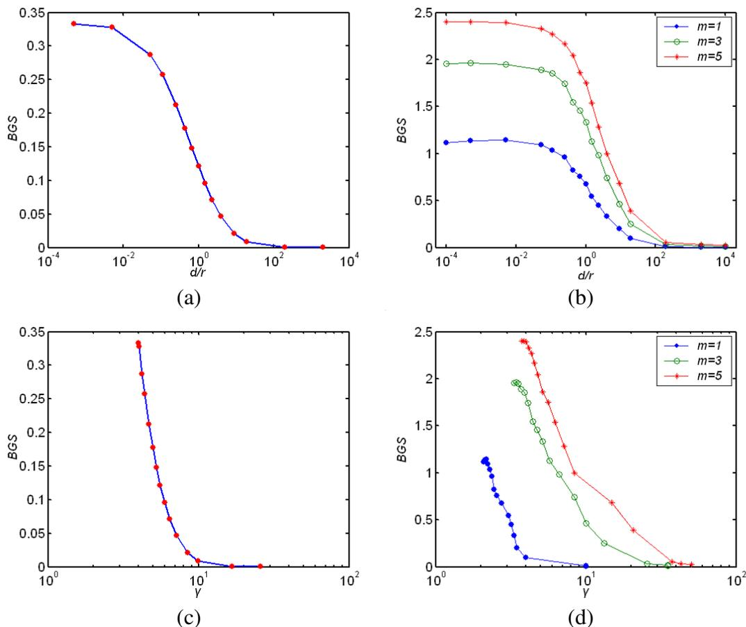
**Figure 2.** *BGS* versus  $d/r$  and  $\gamma$  with network size  $N=2000$ ,  $m=1, 3, 5$ , where (a), (c) are theoretical results for *BGS* and (b), (d) are numerical simulation results respectively.
