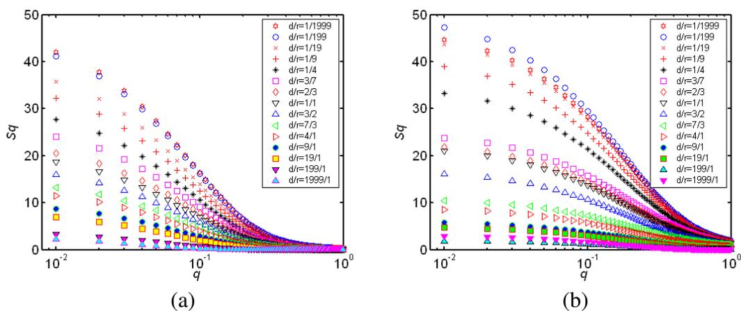
**Figure 3.** The relationship between  $S_q$  and  $q$  under different  $d/r$ ,  $N=2000$ . The  $d/r$  of these plots spans from  $1/1999$  to  $1999/1$ , where (a) is theoretical result and (b) is numerical simulation result.
