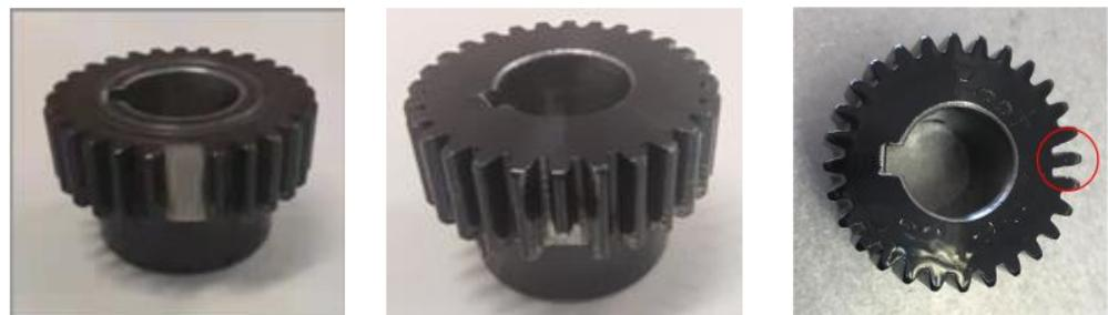
**Figure 2.** Sun gear failure modes (**left**: missing tooth; **middle**: tooth break; **right**: tooth crack).
