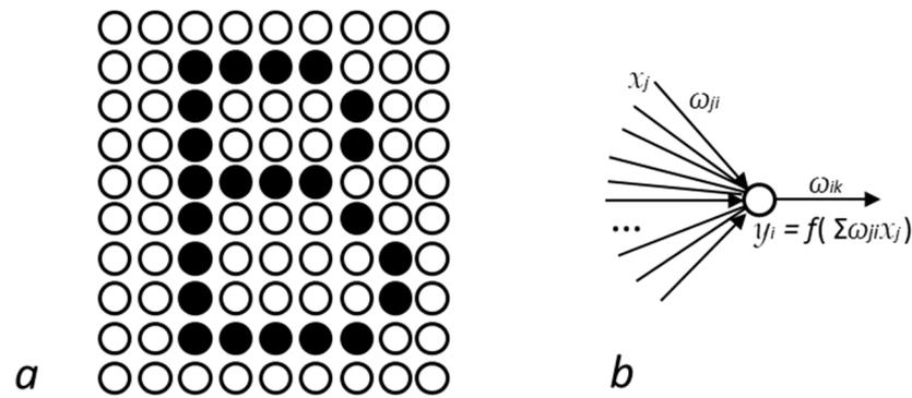
**Figure 4.** (a) Pattern (attractor) memorized in a recurrent neural network. (b) Each neuron receives the weighted signal from all other neurons and emits a signal accordingly.
