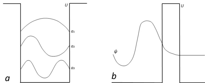
**Figure 3.** (a) Eigenstates in one-dimensional potential well. (b) Tunneling.
