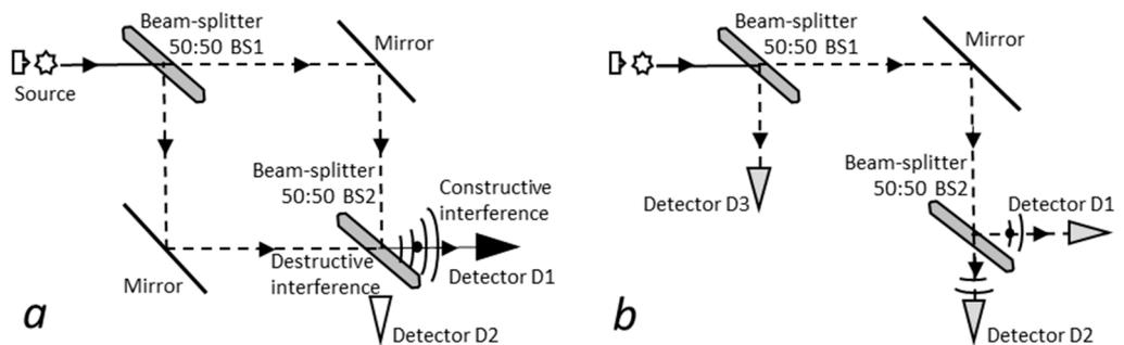
**Figure 1.** Mach-Zehnder interferometer experiment. (a) Interference occurring at beam-splitter BS2 causes particles to be detected only at detector D1. (b) Particles undetected by detector D3 do not undergo interference at BS2 and are detected by both detectors D1 and D2.
