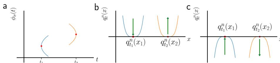
**Figure 5.** (a) Root branches not connected to the boundary  $t = 2$ . As a new feature, the bifurcation at  $t_2$  opens to the left. (b) A first possibility in state space for local extrema of  $q_t^n(x)$  to produce the bifurcations in panel (a). (c) A second possibility in state space for local extrema of  $q_t^n(x)$  to produce the bifurcations in panel (a).
