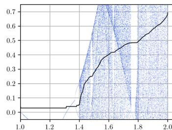
**Figure 7.** Topological entropy of  $q_t$  using the Formula (52) with the logarithm to the base  $e$ . The topological entropy was plotted on the bifurcation diagram for a better understanding of its characteristics.
