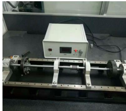
Figure 11. ZHS-5 multi-function rotor experiment bench.
