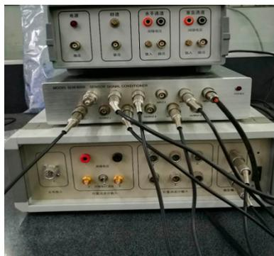
Figure 12. Model SLM-6000 sensor signal conditioner.
