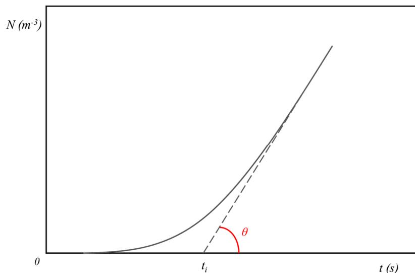
**Figure 1.** Schematic curve of the number of the nuclei density ( $N$ ) as a function of time.  $t_i$  is the induction time and the tangent of  $\theta$  is equal to the nucleation rate in the steady-state ( $I_{st}$ ).
