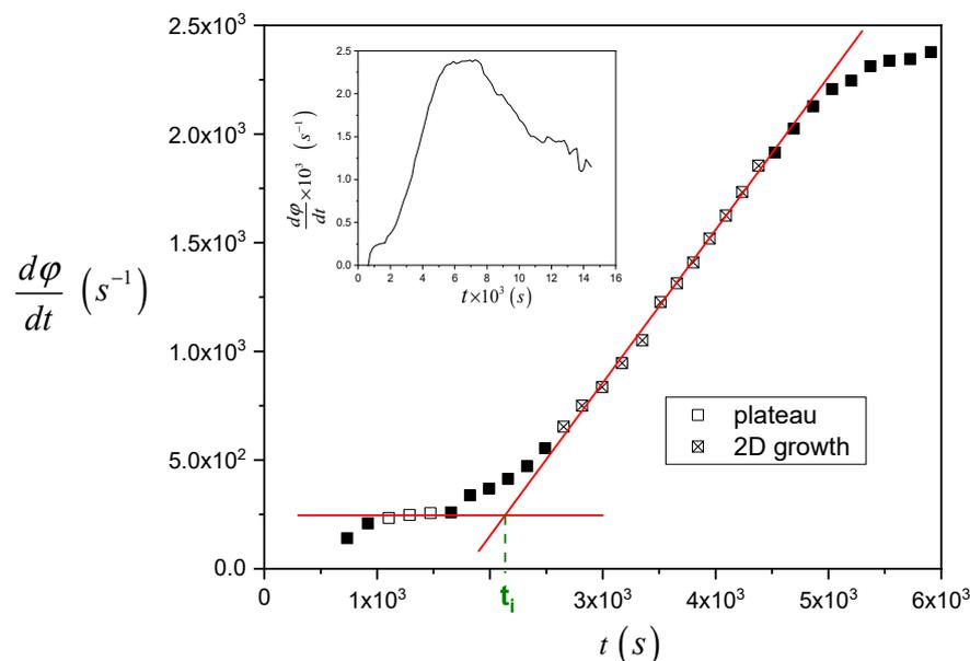
**Figure 5.** Example of the procedure for the calculation of  $t_i$  (the raw data are shown in Figure 4). In the inset plot, the time-derivative of the mean gray value is shown over a more extended time range.
