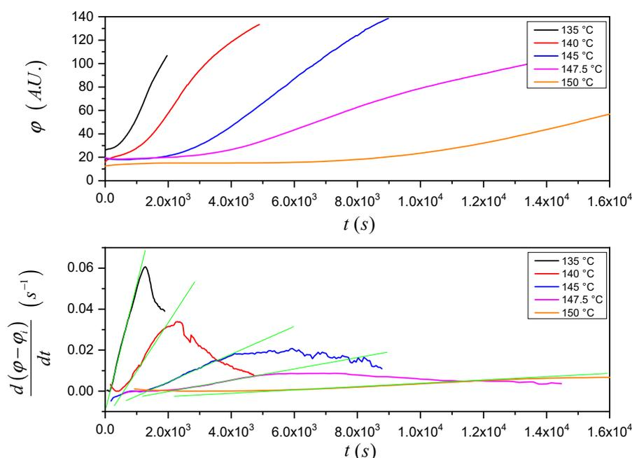
**Figure 6.** Mean gray value as a function of time recorded at the different indicated crystallization temperatures (top) and corresponding time-derivative of the normalized mean gray value vs. time (bottom). The green lines represent the linear fitting of the data in the two-dimensional growth region.
