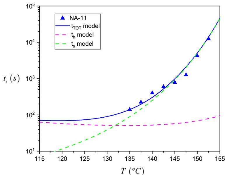
**Figure 11.** Plot of the experimental induction time data at different crystallization temperatures for the iPP/NA-11 system, together with the functions obtained from the fitting of the detailed model for the induction time ( $t_{tot}$ ). The dashed curves represent the contributions of the first layer and further layers formation ( $t_h$  and  $t_s$  models, respectively).
