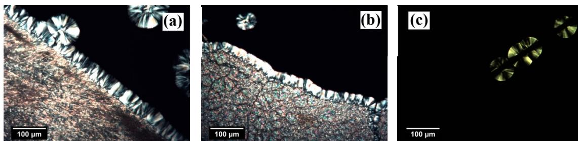
**Figure 2.** Morphologies obtained after isothermal crystallization at 142.5 °C for (a) sodium benzoate (NaBz), (b) sodium 2,2'-methylene bis-(4,6-di-tert-butylphenyl)phosphate (NA-11) and (c) glass fiber (GF). The crystallization times were: (a) 2.0 h, (b) 2.4 h and (c) 1.5 h.
