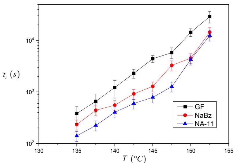
**Figure 7.** Induction time values at different crystallization temperatures for iPP in contact with GF, NaBz and NA-11 (the lines connecting the data of each series are just to guide the eyes). The data reported in the graph are the average of at least three repetitions and the average percent standard deviation is 20% (indicated by the error bars).
