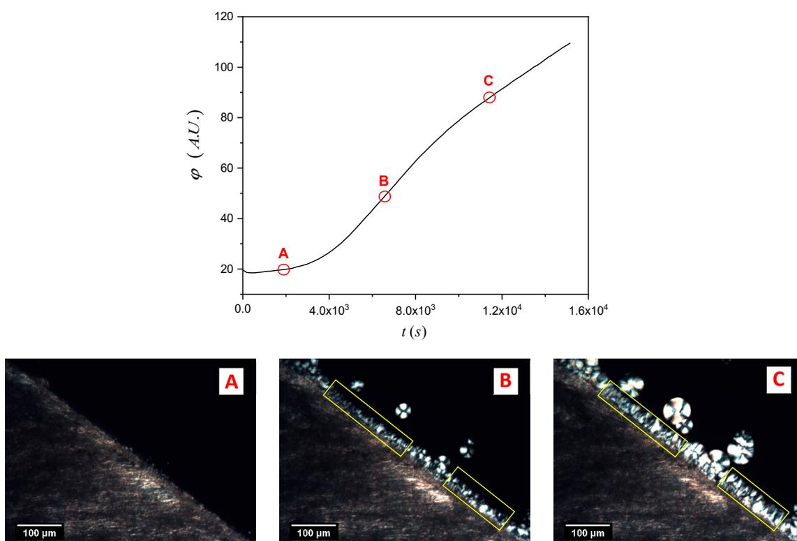
**Figure 4.** Mean gray value ( $\varphi$ ) as a function of time during an isothermal experiment conducted at 147.5 °C for the isotactic polypropylene iPP/NaBz sample. Three micrographs, corresponding to the points A, B and C on the curve, are reported to show the morphological variation. The yellow rectangles indicate the region of interest used to compute the light intensity.
