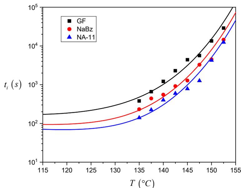
**Figure 10.** Plot of the induction time data as a function of crystallization temperature for the three systems, with the best fitting functions represented by the continuous lines and obtained through the simultaneous fitting of the detailed model (Equation (8)) on all experimental data.
