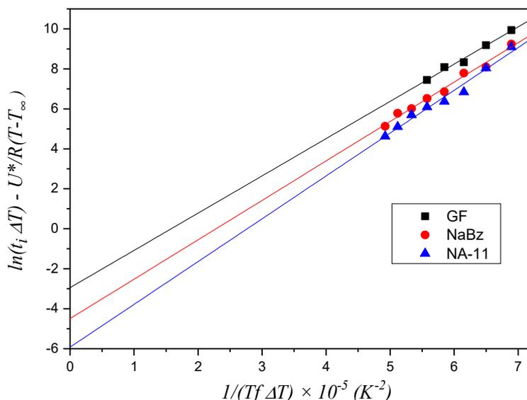
**Figure 9.** Plot of the experimental induction time data of the three systems according to the further layers method (Equation (3)). The constant values employed for  $U^*$  and  $T_\infty$  are reported in Table 2, while the value of  $T_m^\circ$ , equal to 188 °C (461.15 K), was obtained from the best fit of the data.
