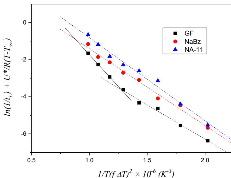
**Figure 8.** Plot of the experimental induction time data of the three systems according to the first layer model (Equation (2)). The constant values employed for  $U^*$  and  $T_\infty$  are reported in Table 2, while the value of  $T_m^\circ$ , equal to 188 °C (461.15 K), was obtained from the best fit of the data.
