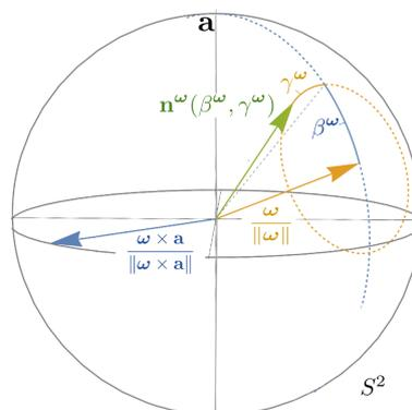
**Figure 2.** For  $\omega \neq \mathbf{a}$ , we parameterize every orientation  $\mathbf{n}$  (green) by rotations around  $r^{-1}\omega$  (orange) and  $\frac{\omega \times \mathbf{a}}{\|\omega \times \mathbf{a}\|}$  (blue). In other words,  $\mathbf{n}^\omega(\beta^\omega, \gamma^\omega) = \mathbf{R}_{r^{-1}\omega, \gamma^\omega} \mathbf{R}_{\frac{\omega \times \mathbf{a}}{\|\omega \times \mathbf{a}\|}, \beta^\omega}(r^{-1}\omega)$ .
