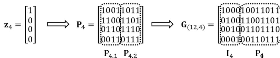
Figure 1. A generator matrix of the  $(12, 4)$  BLRCs in Construction 1.
