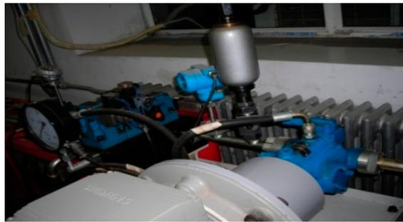
Figure 12. Experimental test rig of SCY hydraulic plunger pump.
