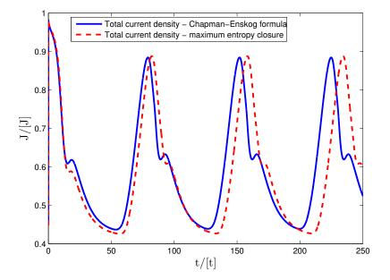
**Figure 2.** Nondimensional current density versus time from the current balance equation obtained by using the Chapman–Enskog (solid line) and the maximum entropy closure (dashed line). Current density and time scales are as in Table 1 for a DC voltage bias of 1.5312 V.
