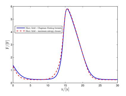
**Figure 3.** Nondimensional field profile at the same instant of an oscillation period from the current balance equation obtained by using the Chapman–Enskog (solid line) and the maximum entropy closure (dashed line). Field and space scales are as in Table 1 for a DC voltage bias of 1.5312 V.
