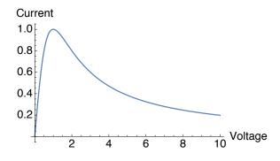
**Figure 1.** Nondimensional current–voltage characteristic curve J(F) for constant field and current density. Up to order  $\lambda^2$  terms, it is the same whether we use maximum entropy closure or the Chapman–Enskog formula derived below.
