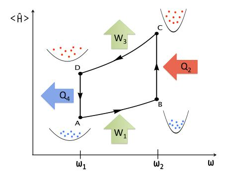
**Figure 1.** Many-particle quantum heat engine. Quantum Otto cycle with a quantum fluid as a working medium confined in a harmonic trap with frequency varying between  $\omega_1$  and  $\omega_2$ . States at A and C are thermal, while those at B and D are generally nonequilibrium states.
