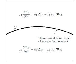
Figure 2. A contact surface  $\Sigma$  having its own physical characteristics.
