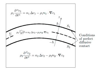
Figure 1. Thin intermediate layer between two media.
