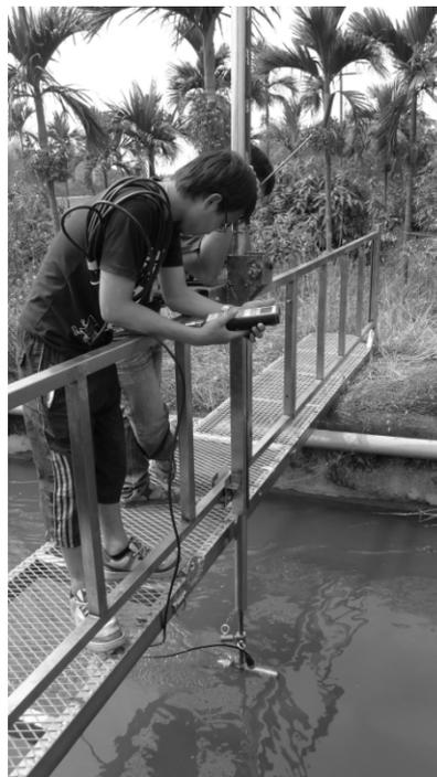
The Wan-Dan Canal is a 3 m wide rectangular channel built with reinforced concrete. To develop a reliable and accurate discharge measurement method for the Wan-Dan Canal, a large amount of data on velocities over the full cross-section is collected. It is conventional to make the nine verticals
