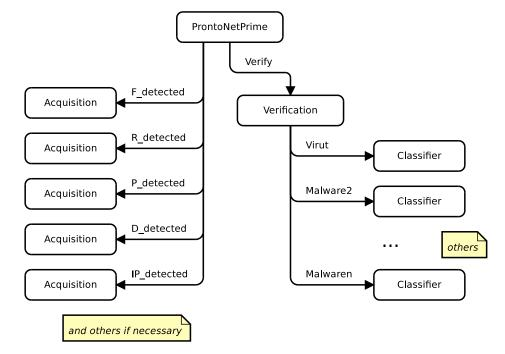
The hierarchical structure of the CP-net model defined by the authors is shown in Figure 1. The detection process progresses on the basis of the levels of the hierarchy. The primary module of the CP-net
