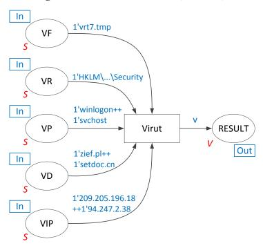
In the presented example, assuming the appearance of the appropriate marking, transition Virut is enabled, which, as a consequence, leads to receiving vector v informing about detection of the Virut malware. The structure of vector v is as follows:
