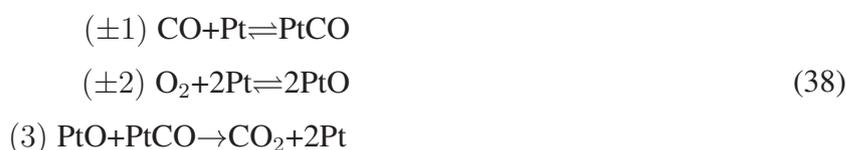
The kinetic equations for this system (including the flux in the gas phase) is
