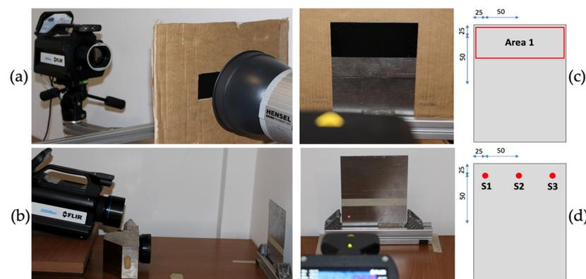
**Figure 1.** Experimental set up in (a) transmission mode, and (b) reflection mode. Scheme of the inspected areas for (c) transmission and (d) reflection measurements (lengths are in mm).
