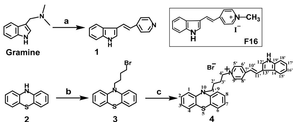
**Scheme 1.** Synthesis of conjugate 4: (a) pyridinecarboxaldehyde, *N*-butyl phosphorus,  $CH_3CN$ , 60 °C, 24 h; (b) 1,4-dibromobutane, NaH, 0 °C, 1 h; (c) **1**, DMF or  $CH_3CN$ , 85 °C, 16 h.
