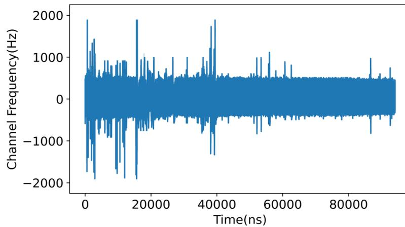
Figure 6. Channel frequency after wavelet transform.
