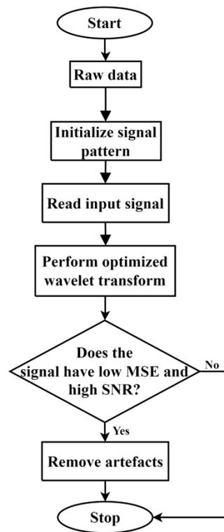
**Figure 3.** Flow chart of optimized wavelet transform.
