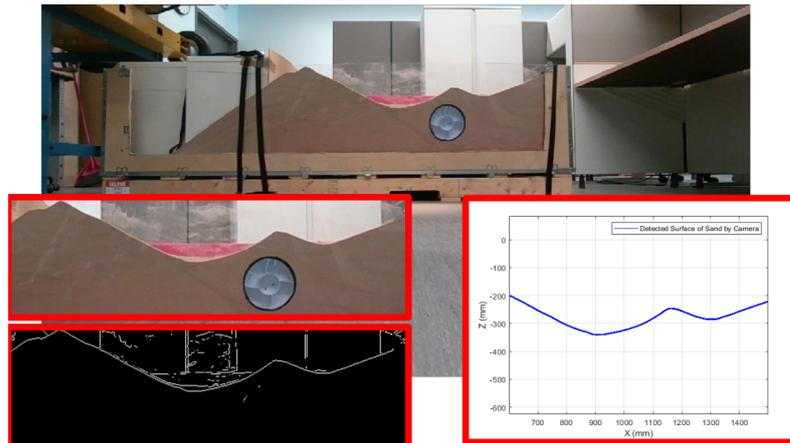
**Figure 13.** Detecting ground shape using RGB camera and MATLAB R2021a software.
