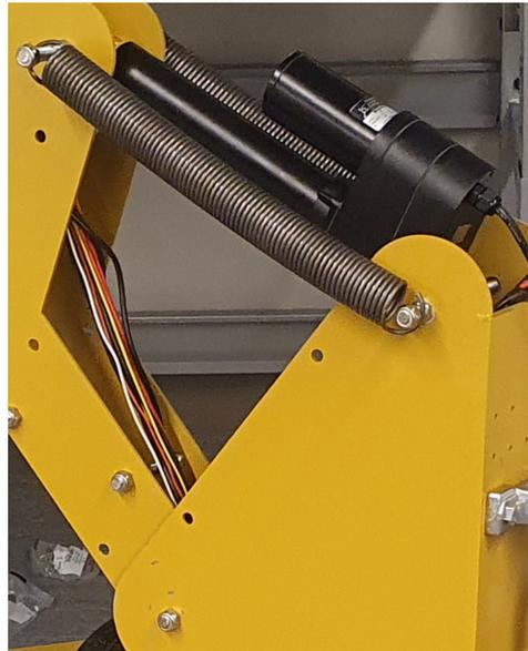
**Figure 7.** Two massive springs helping the boom actuator raise the manipulator.
