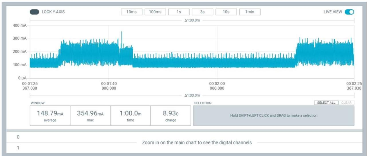
Figure 17. Current consumption with NB-IoT, BLE Mesh, sensors and GPS turned on [36].
