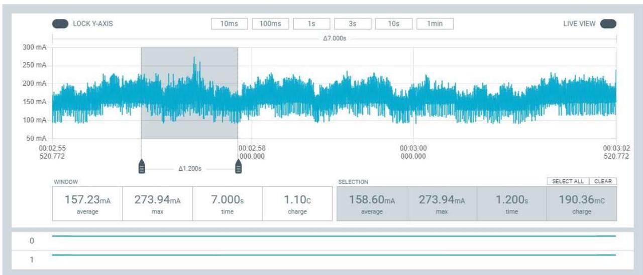
**Figure 19.** Current consumption during BLE Mesh usage [36].
