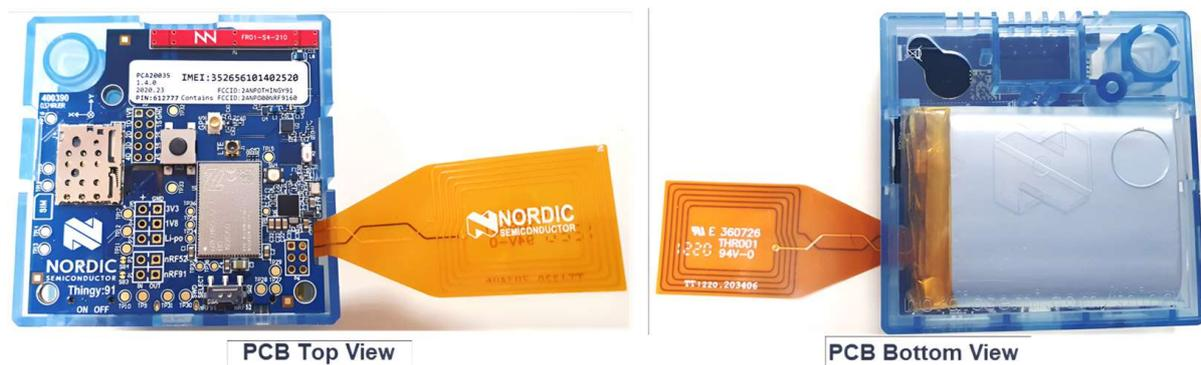
Figure 5. The purchased Nordic Thingy:91 prototyping platform [31].
