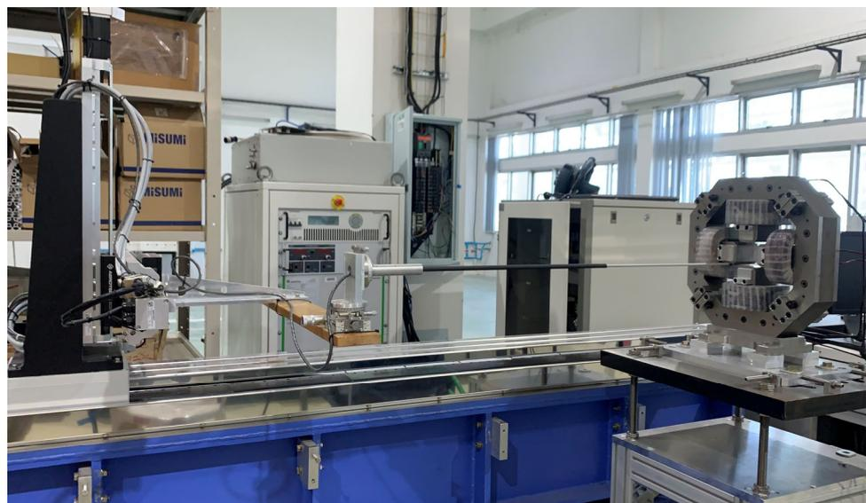
**Figure 9.** Hall probe bench for magnetic field measurement.
