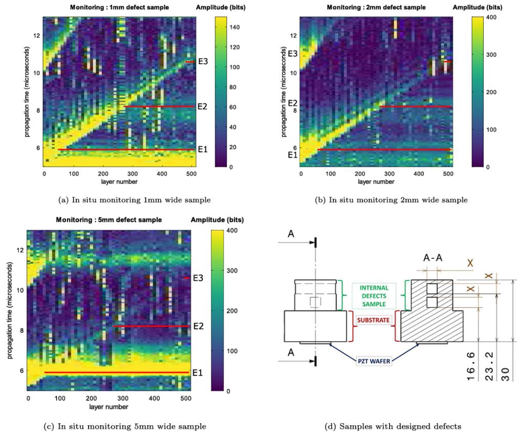
**Figure 14.** In situ monitoring of samples with internal designed defects [38].
