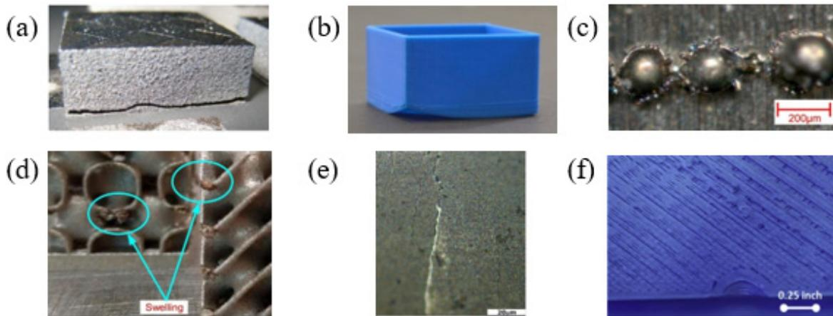
**Figure 1.** Typical examples of defects in additive manufacturing showing: macro-cracks (a) [23], warping (b) balling (c) [24], swelling (d) [25], micro-cracks (e) [26], and an under-filled part (f) [27].
