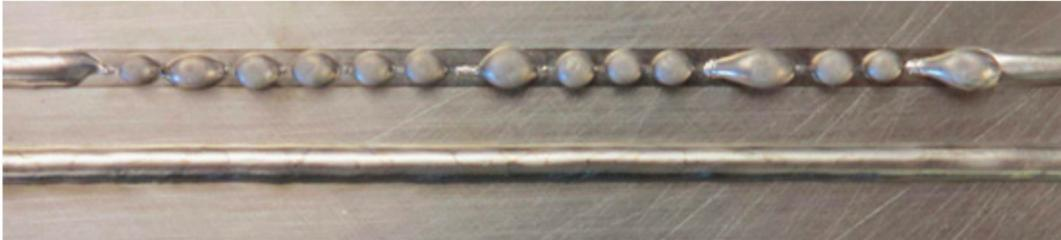
**Figure 33.** Top track deposited without employing a controller. The bottom track deposited utilizing a controller for adjusting the position of the deposition head in the Z direction (reproduced with permission from [97]: copyright 2014, Elsevier Ltd.).
