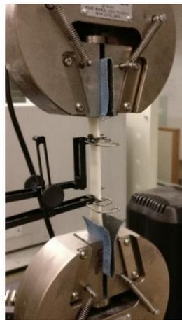
Figure 5. Tensile testing setup.
