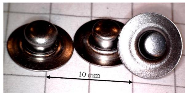
**Figure 1.** ECG studs produced by micro-sheet forming.
