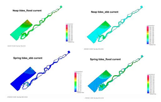
Figure 5. Maps of current velocity simulated during spring and neap tides on April 2021 (Food/ebb).
