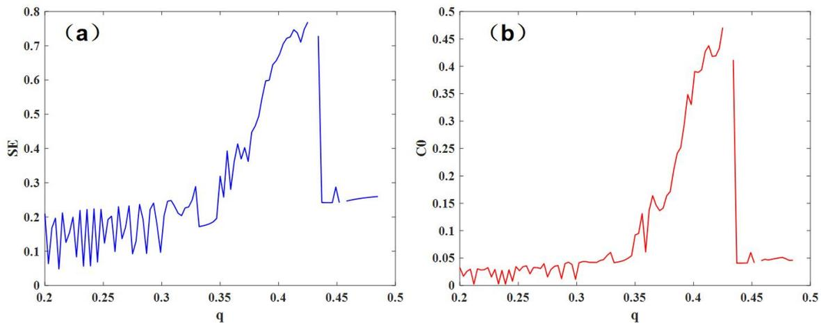
**Figure 7.** System complexity when  $q$  changes: (a) SE complexity; (b) C0 complexity.
