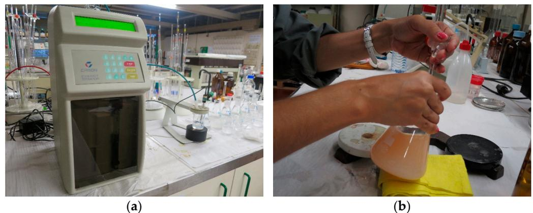
**Figure 3.** The main steps of chloride content determination: (a) free chloride and (b) total chloride.
