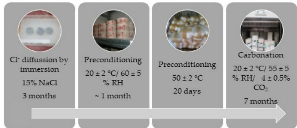
Figure 4. Scheme for combining tests to study the effect of the presence of chlorides on carbonation.
