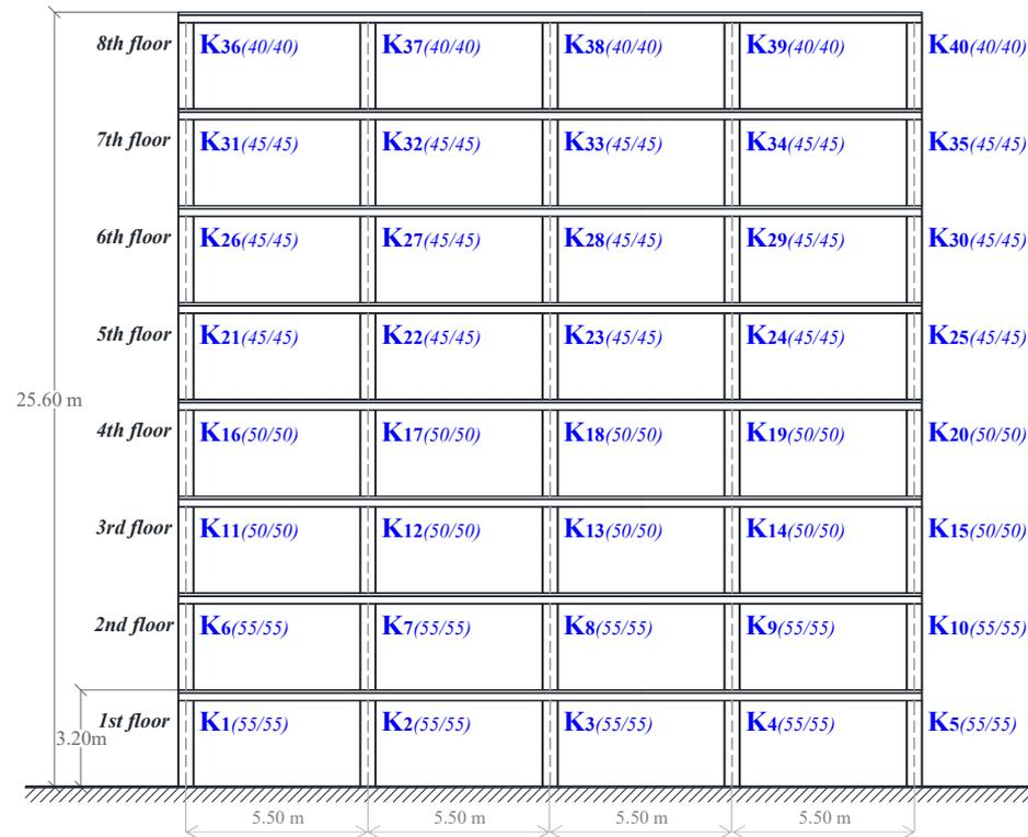
Figure 2. Examined 8-storey RC frame structure.
