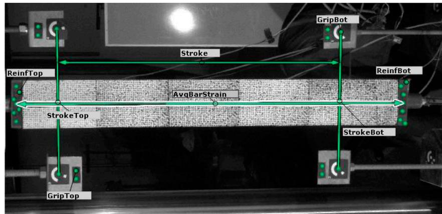
Figure 7. Installed specimen on uniaxial testing machine with defined components.
