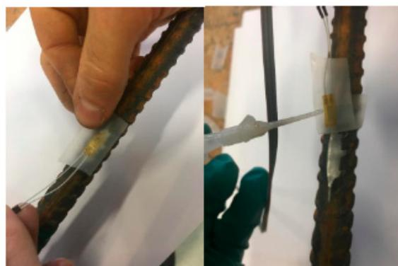
Figure 5. Installing SGs on rebars.
