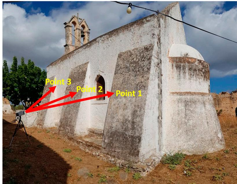
**Figure 7.** The first station of the laser scanning head at the south side of the chapel and the first three laser spot target points.
