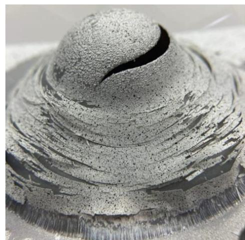
**Figure 17.** Separated paint after forming as shown for P7/SC4, P4/SC1.
