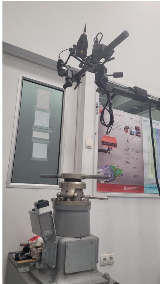
**Figure 10.** Erichsen testing equipment with GOM ARAMIS 5M DIC system (own photo).
