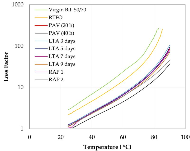
Figure 6. Loss factor versus temperature curve.
