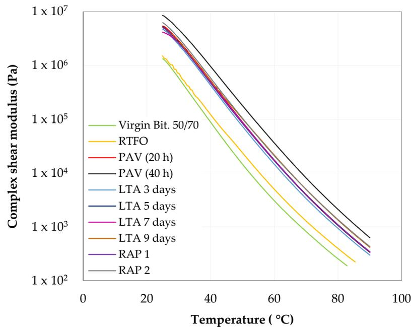
Figure 7. Isochronal plots of the complex shear modulus ( $G^*$ ).
