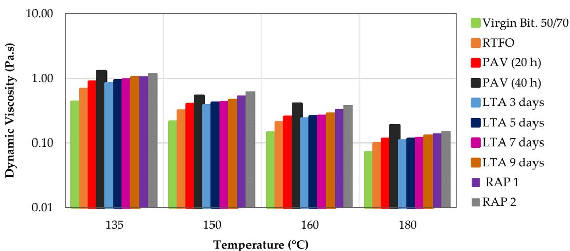
Figure 5. Dynamic viscosity of the aged binders over various temperatures.
