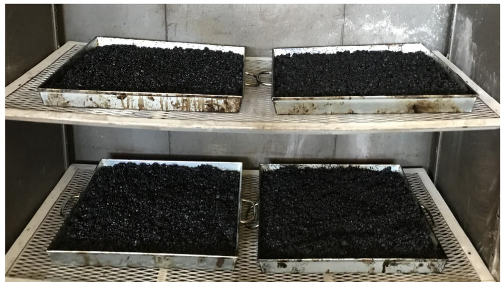
**Figure 2.** Loose asphalt mixture oven ageing.
