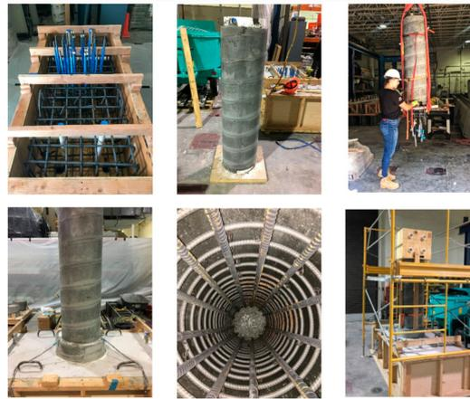
Figure 6. Construction steps for the first specimen.
