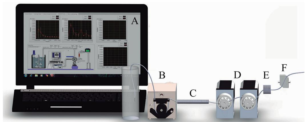
**Figure 1.** Main components of the SIA System with UV/visible spectrophotometer; (A) graphical user interface, (B) peristaltic pump, (C) holding coil, (D) multiposition valves, (E) reaction coil, and (F) flow cell.
