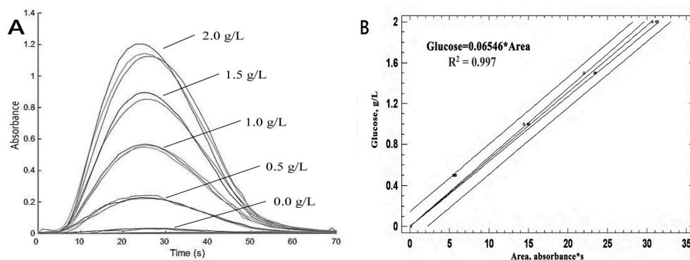
**Figure 6.** Response from SIA: (A) response of the SIA system in front of different substrate concentrations; (B) calibration curves.
