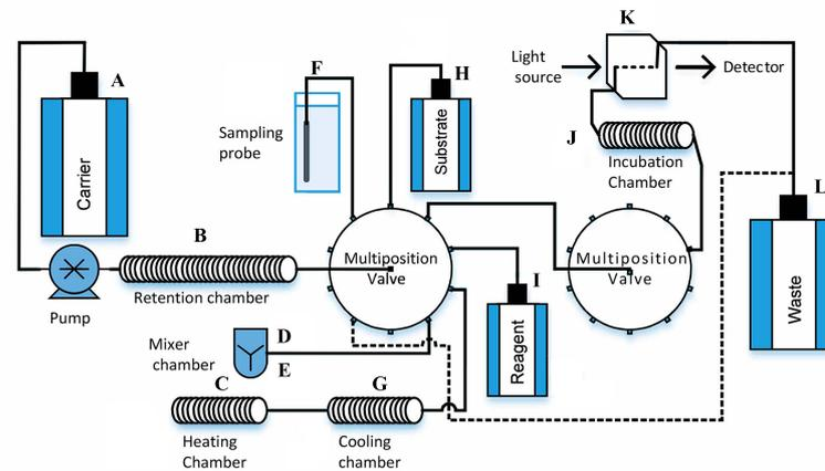
**Figure 2.** Specific components of the lab-made model used to determine  $\beta$ -fructofuranosidase activity. (A) Carrier, (B) retention chamber, (C) heating chamber, (D,E) mixer chambers, (F) bioreactor and sampling probe, (G) cooling chamber, (H) substrate, (I) reagents, (J) incubation chamber, (K) spectrophotometric detector, and (L) waste container.
