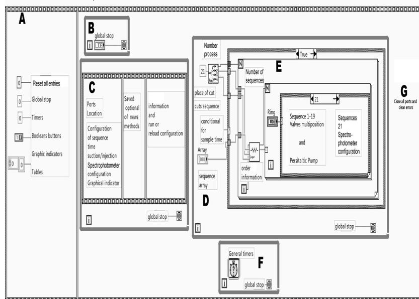
**Figure 4.** Virtual code to control the overall components of the SIA system. (A) initialization, (B) global stop, (C) USB port configuration, (D) control of the actuators, (E) sequences to activate components, (F) control of the sample, and (G) saving data.
