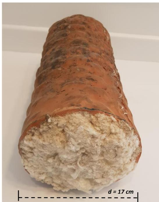
**Figure 1.** Oil and gas mooring line used in this work, which is made of polyamide fibers (PAF).
