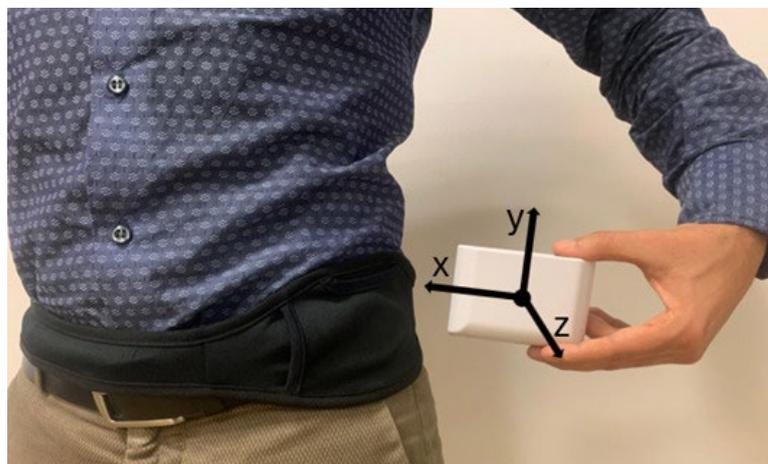
**Figure 1.** Wearable sensor (STAT-ON™) position and axes orientation.
