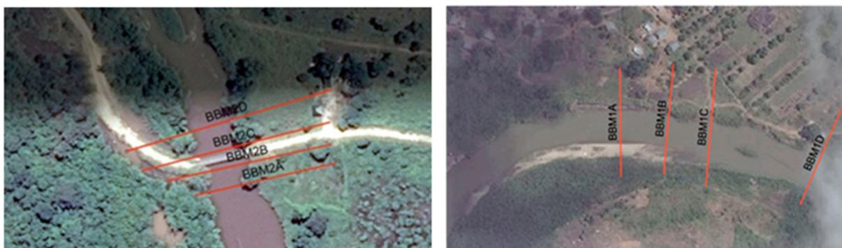
**Figure 2.** Channel cross-section depth survey transects at Gama Gate (left) and Matipwili (right), Wami River, Tanzania.
