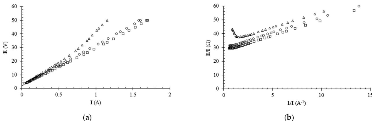
**Figure 2.** Voltage-current (E-I) curves (a) and corresponding Cowan and Brown plot (b) for aqueous citric acid solutions at three different citric acid concentrations ( $\Delta = 0.9 \text{ g/L}$ ;  $\circ = 3.7 \text{ g/L}$ ;  $\square = 23.9 \text{ g/L}$ ).
