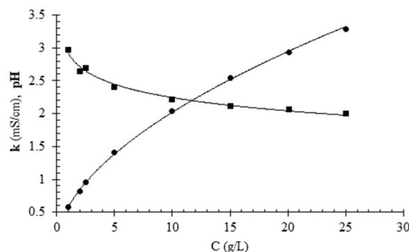
**Figure 1.** Electric conductivity  $k$  (●) and pH (■) at 20 °C of citric acid aqueous solutions as a function of citric acid concentration (C). The symbols refer to experimental data while the continuous lines refer to approximating curves.
