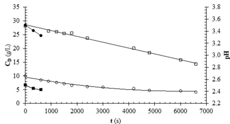
**Figure 5.** Time course of pH ( $\bullet$ ,  $\circ$ ) and titratable acidity concentration ( $C_D$ ) ( $\blacksquare$ ,  $\square$ ) for the deacidification of pineapple juice carried out at  $I = 0.75$  A as such (closed symbols) or at  $I = 1$  A enriched with approximately 20 g/L of citric acid (open symbols).
