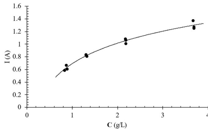
**Figure 3.** Limiting current intensity ( $I_{lim}$ ) vs. solution citric acid concentration (C). The symbols refer to experimental data while the continuous lines refer to the approximating curve.
