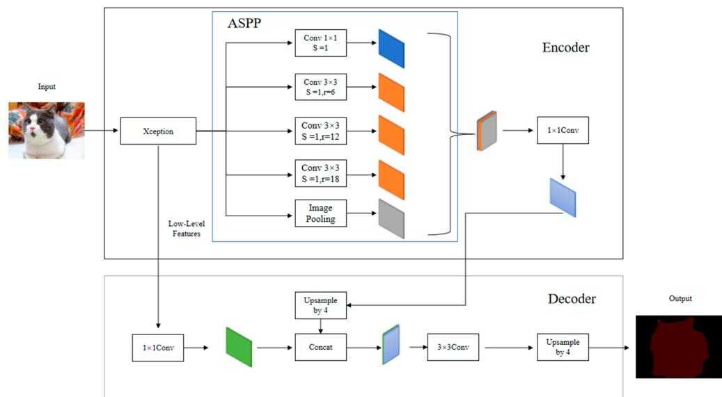
**Figure 2.** DeepLabV3+ benchmark network structure.
