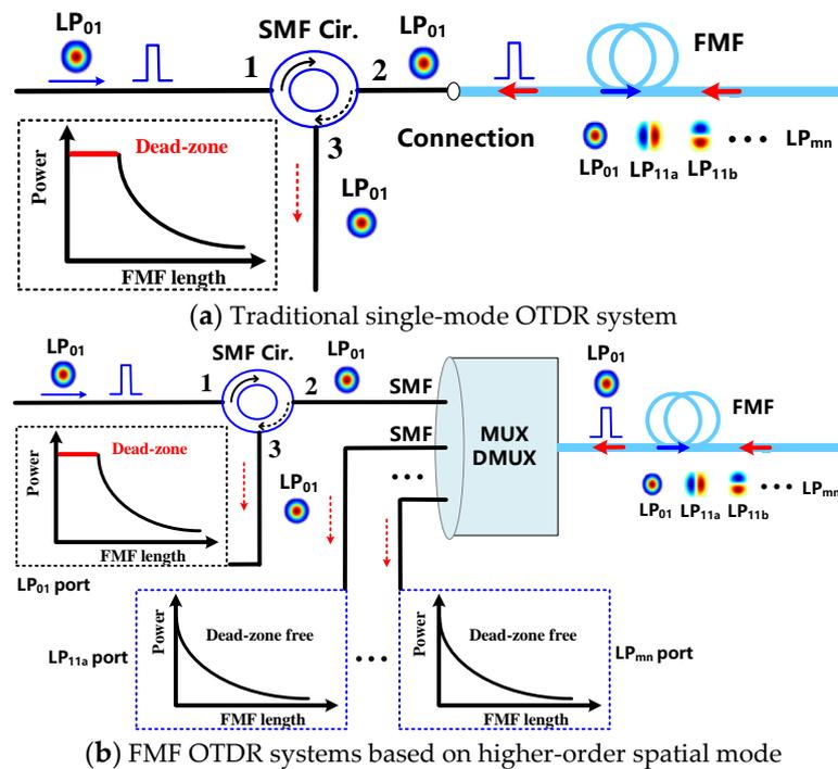
**Figure 1.** Principle comparison between traditional single-mode OTDR and FMF OTDR based on the higher-order spatial mode.
