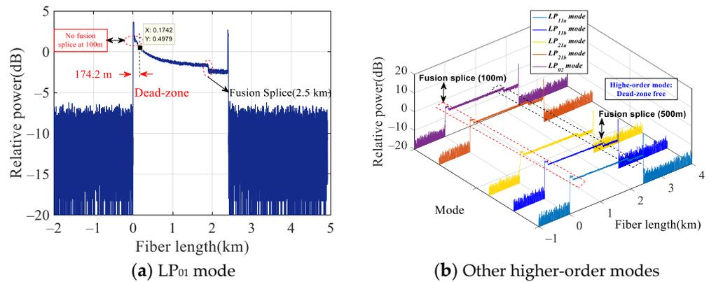
**Figure 6.** The detection results of the fusion splice located at 100 m under the condition of the 100 ns probe optical pulse.
