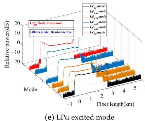
**Figure 7.** Dead-zone-free detection results of fusion splice faults based on FMF OTDR under different excitation modes.
