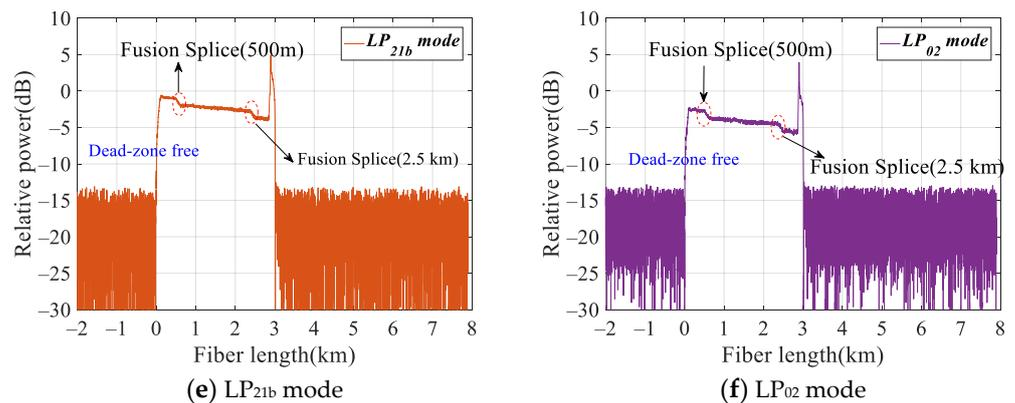
**Figure 5.** The detection results of the fusion splice fault, dead-zone-free, based on the higher-order spatial mode OTDR.
