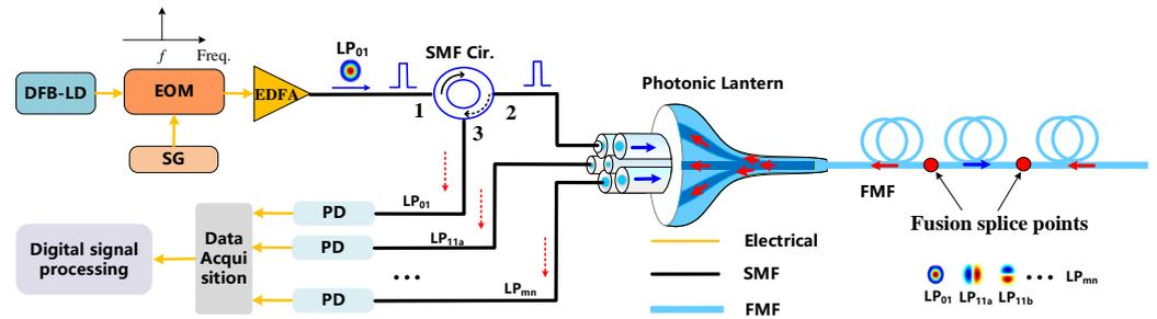
**Figure 4.** Experimental setup for dead-zone-free fault detection of an FMF link based on higher-order spatial mode Rayleigh backscattering.
