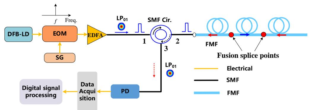
Figure 2. FMF link fault detection experimental setup based on traditional single-mode OTDR.
