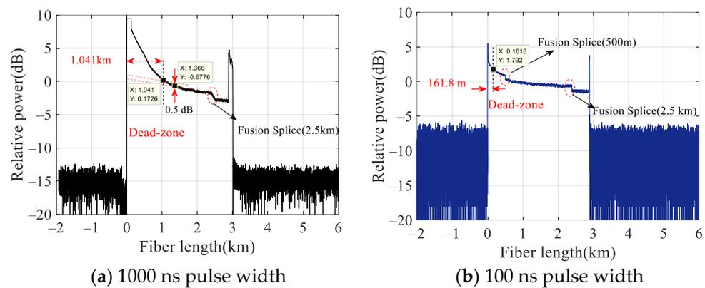
**Figure 3.** Detection results of fusion faults in the FMF link based on the traditional single-mode OTDR under different optical pulse widths.
