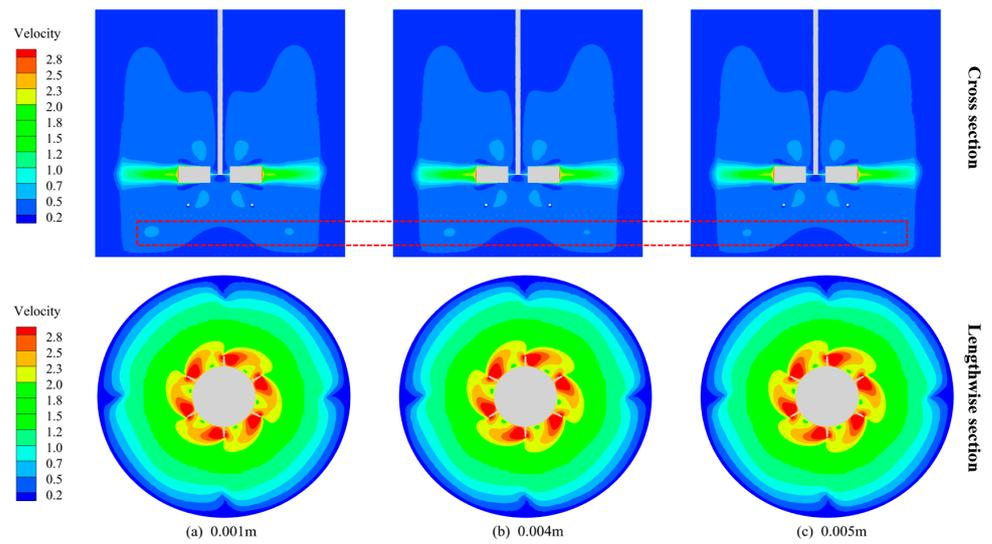
**Figure 19.** Velocity distribution inside the stirred tank at different bubble diameters.
