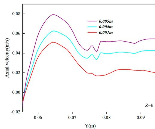
**Figure 21.** Axial velocity distribution of the gas phase in Y direction at  $Z = 0$  in a stirred tank with different bubble diameters.
