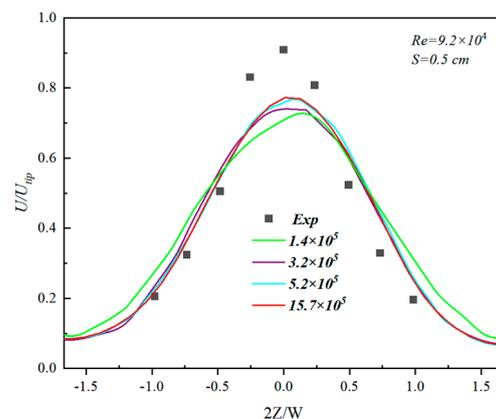
Figure 3. Grid independence study for normalized liquid velocity.
