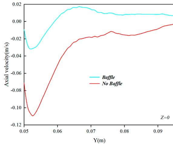
**Figure 14.** Liquid-phase axial velocity distribution in the Y direction at  $Z = 0$  in the stirred tank with or without baffles.
