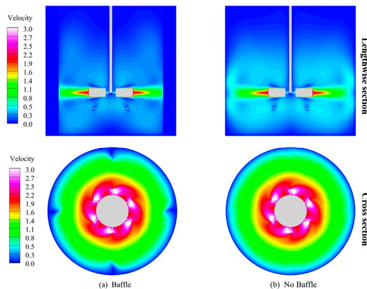
**Figure 13.** Velocity distribution inside the stirred tank with or without baffles.
