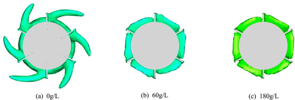
**Figure 10.** Equivalent plots of 0.018 gas holdup behind the impeller in stirred tanks with different sulfuric acid concentrations.
