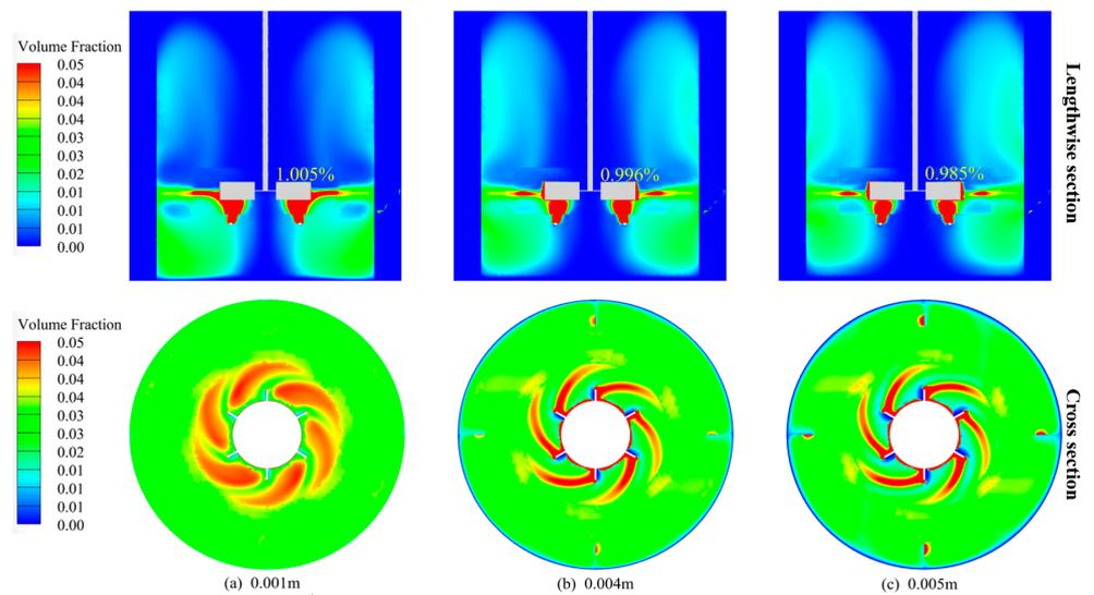
**Figure 20.** Gas holdup distribution inside the stirred tank at different bubble diameters.
