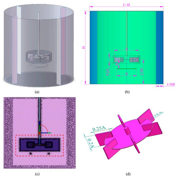
**Figure 1.** (a) Computational domain. (b) Schematic diagram of the stirred tank. (c) Structured grid. (d) Rushton turbine.
