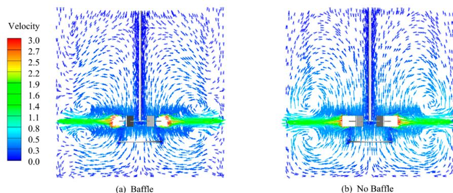
**Figure 11.** Velocity vector inside the stirred tank with and without baffles.
