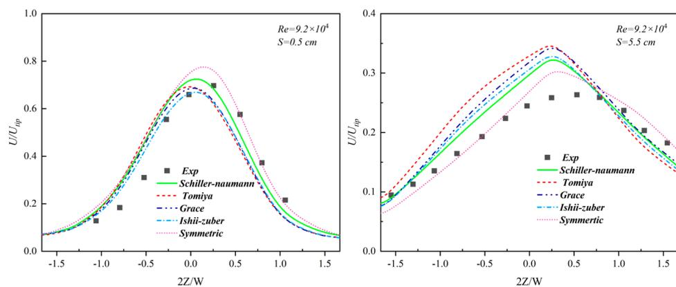
**Figure 6.** Axial distribution of normalized liquid-phase velocity in the drainage zone under different drag force models.
