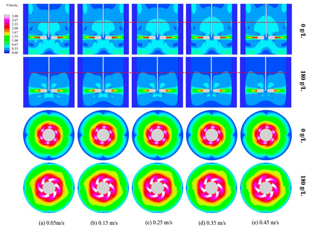
**Figure 22.** Comparison of velocity distribution clouds for different sulfuric acid concentrations at the same inlet velocity in a stirred tank.
