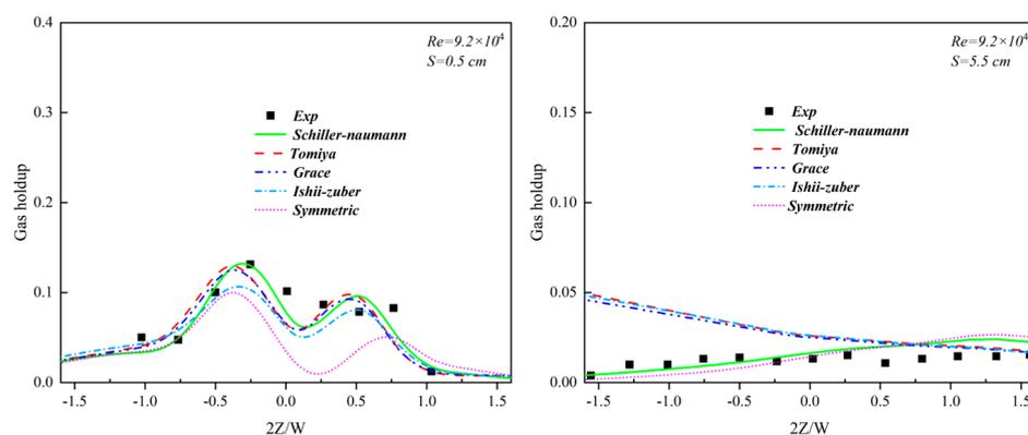
**Figure 7.** Axial distribution of the gas holdup in the drainage area under different drag force models.
