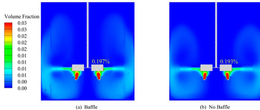
**Figure 12.** Gas holdup distribution inside the stirred tank with and without baffles.
