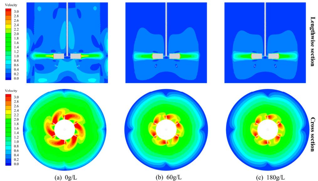
**Figure 8.** Velocity distribution inside the stirred tank under different concentrations of sulfuric acid.
