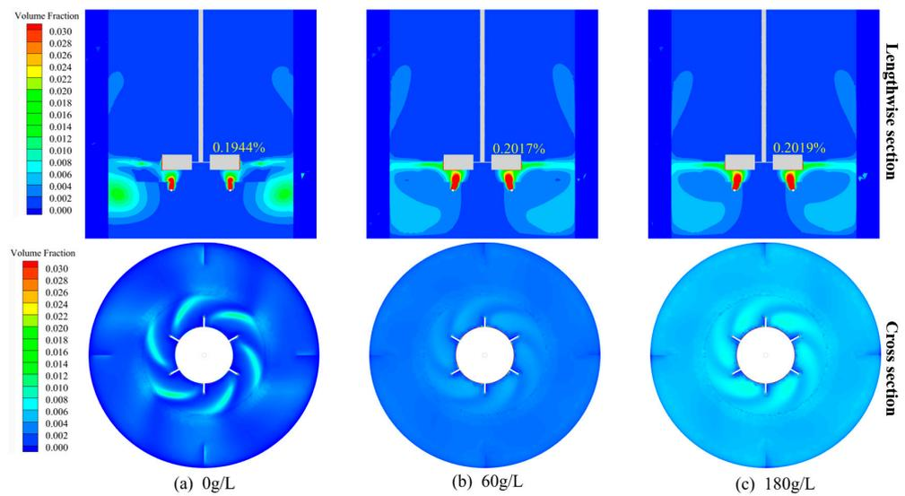
**Figure 9.** Gas holdup distribution inside the stirred tank under different concentrations of sulfuric acid.
