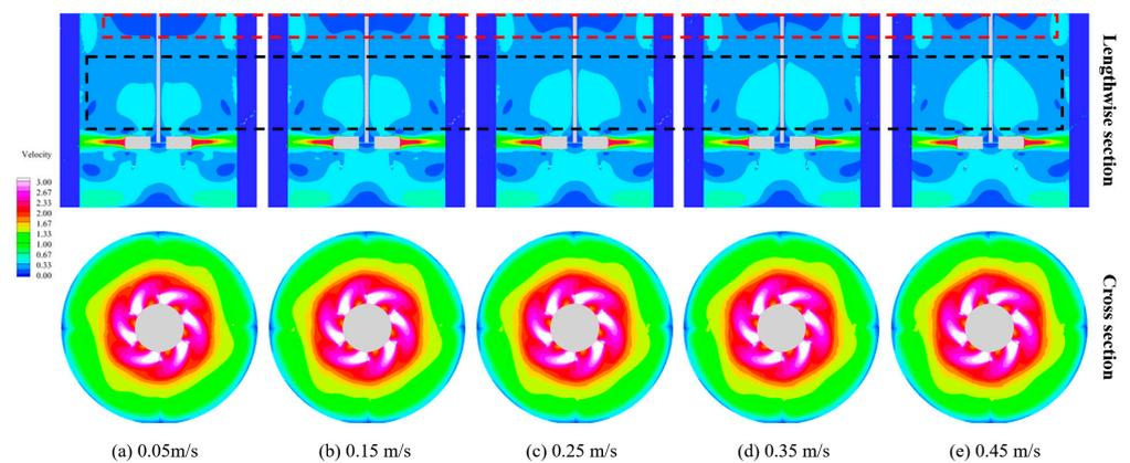
**Figure 16.** Velocity distribution in the stirred tank at different inlet velocities.
