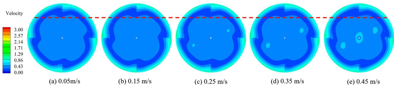
**Figure 17.** Velocity distribution in the stirred tank at different inlet velocities for  $Z = 0.144$  plane.
