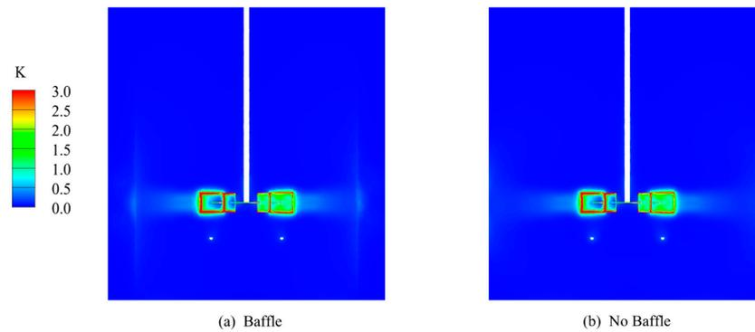
**Figure 15.** Distribution of turbulent kinetic energy inside the stirred tank with or without baffles.
