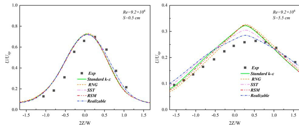
**Figure 4.** Axial distribution of liquid-phase velocity in the discharge zone under different turbulence models.
