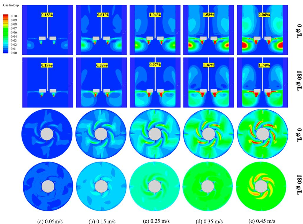
**Figure 23.** Distribution of gas holdup in stirred tanks with different inlet velocities at different sulfuric acid concentrations.
