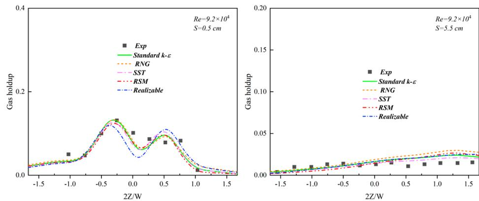
**Figure 5.** Axial distribution of gas holdups in the drainage area under different turbulence models.
