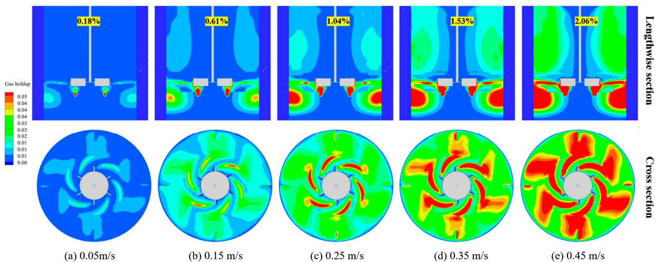
**Figure 18.** The gas holdup distribution inside the stirred tank at different air inlet velocities.
