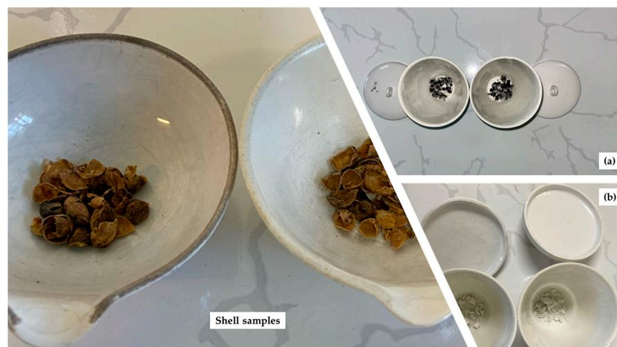
**Figure 4.** Shell samples for analysis: (a) ceramic crucibles after volatile matter content determination and (b) ceramic crucibles after ash content determination.
