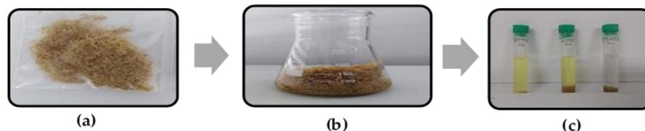
**Figure A1.** (a) Coconut cellulose, (b) cellulose quaternization, and (c) cellulose and cellulose-modified tartrazine.
