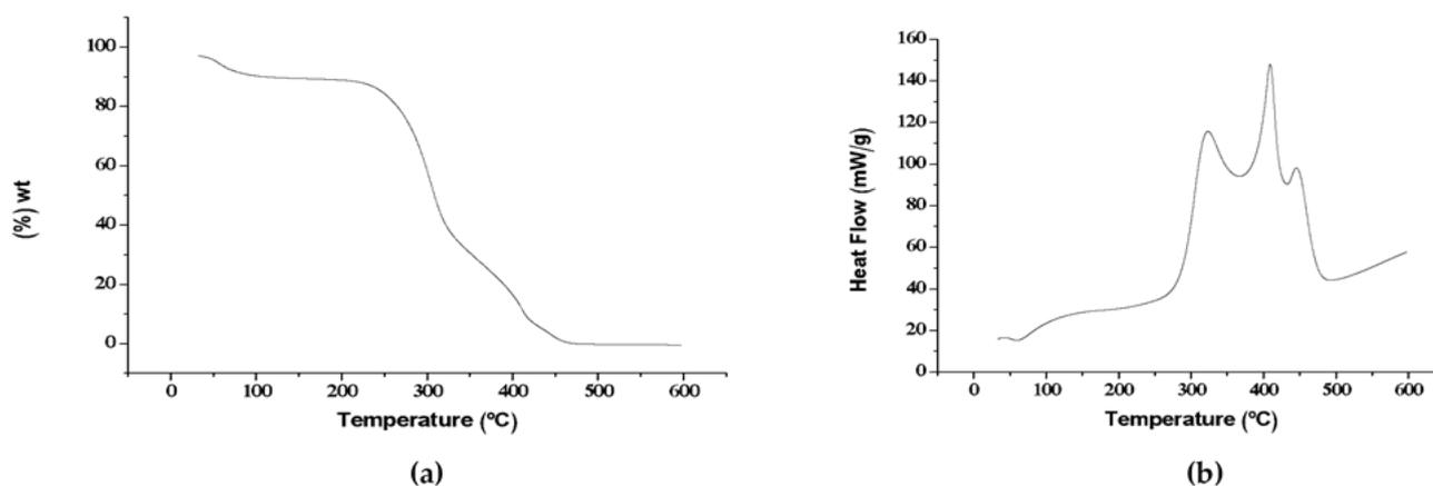
**Figure 2.** (a) TGA and (b) DSC analysis of cellulose extracted from coconut shell.
