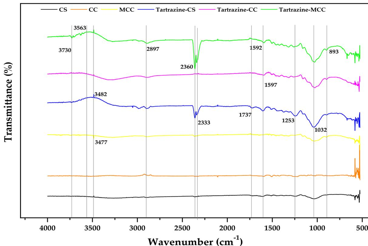
**Figure 3.** Normalized FTIR spectra of coconut-shell-based bioadsorbents before and after tartrazine removal.
