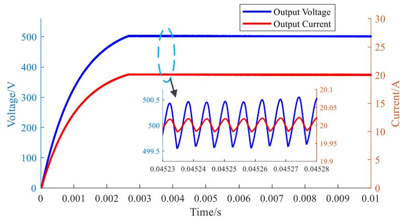
Figure 11. System output voltage and current waveforms during soft startup.
