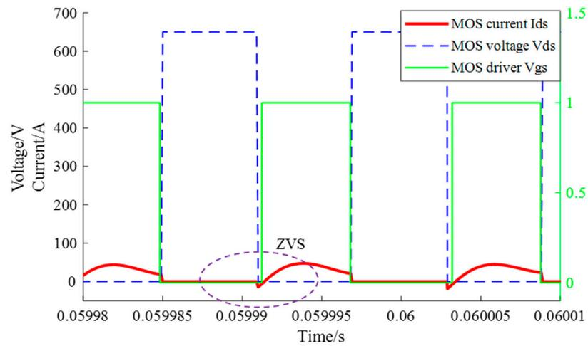
Figure 12. The ZVS waveforms of the rectifier MOSFETs.
