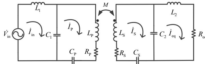
Figure 3. Equivalent circuit of the DLCC IPT system.
