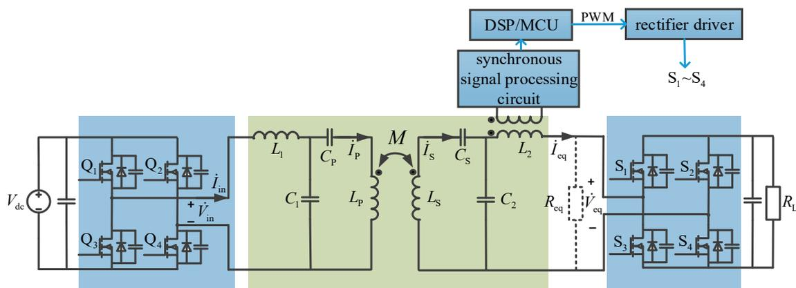
**Figure 2.** Topological structure diagram of the circuit.
