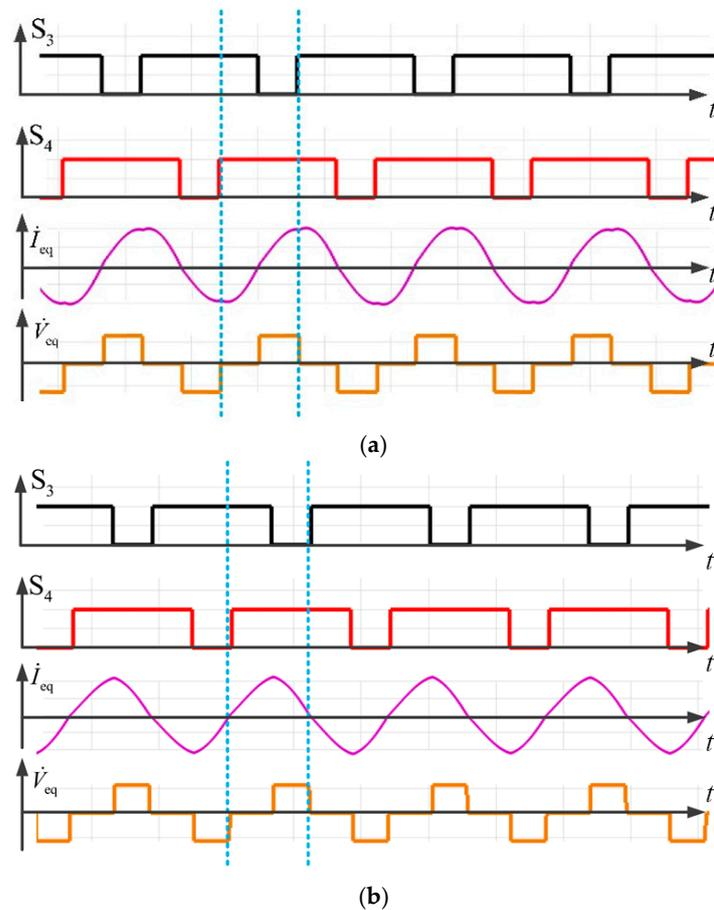
Figure 5. Driving waveforms of the switches and output voltage and current waveforms of the compensation network in two modes. (a) Hard switching mode. (b) Soft switching mode.
