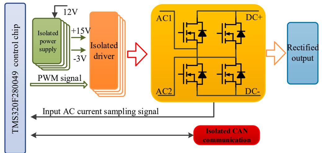
Figure 9. Power block diagram of the synchronous rectifier.
