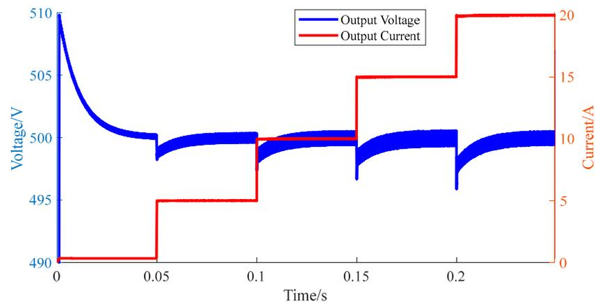
Figure 13. System output voltage and current waveforms during the four-stage loading process.
