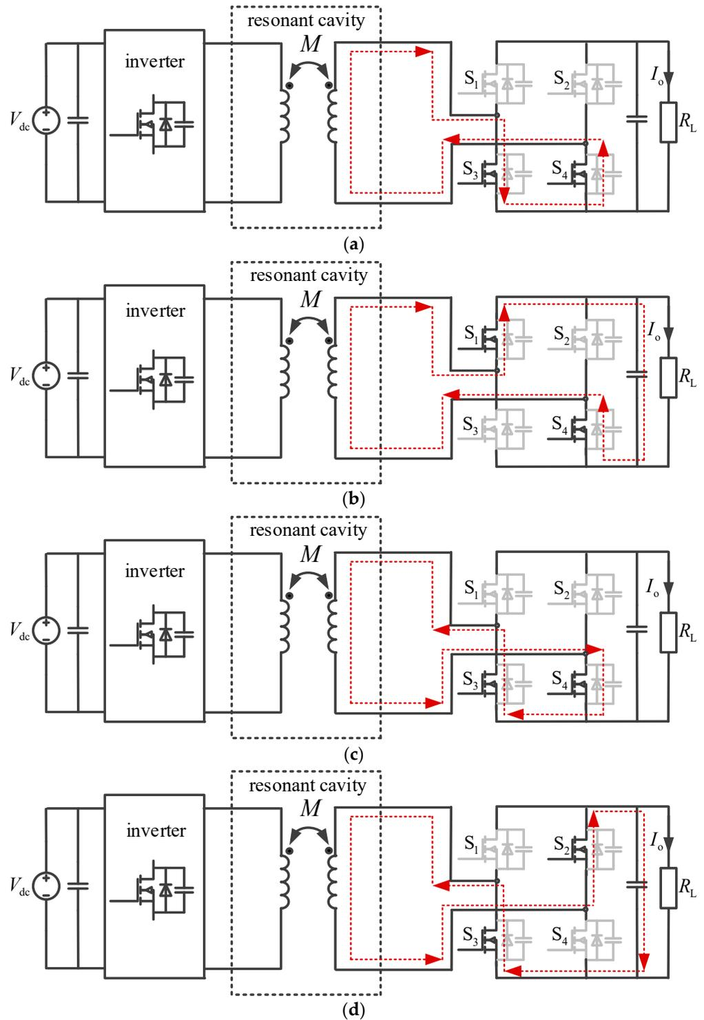
**Figure 7.** Current paths of the four operating modes. (a) Mode I. (b) Mode II. (c) Mode III. (d) Mode IV.
