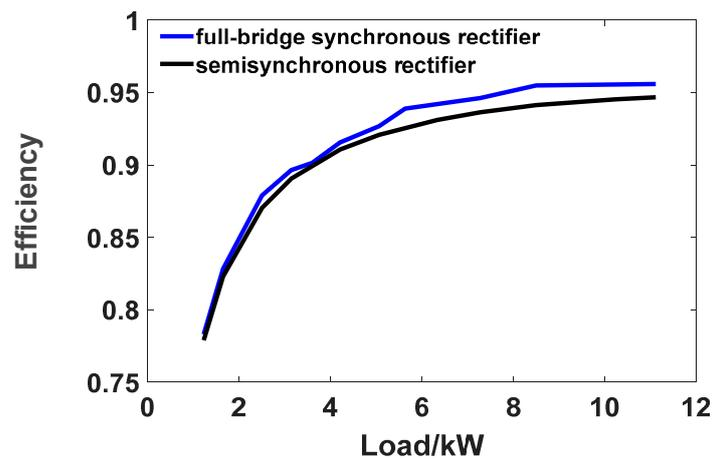
Figure 18. System efficiency diagram at different loads.
