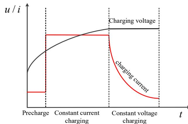
**Figure 1.** Charging curve of the lithium battery.
