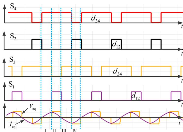
Figure 6. Driving waveforms of the switches and output voltage and current waveforms of the compensation network.
