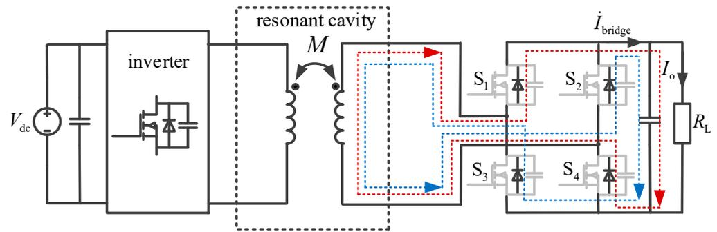
Figure 4. Current path diagram of the rectifier circuit.
