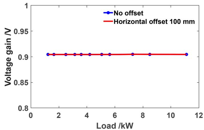
Figure 17. Voltage gain diagram at different loads.
