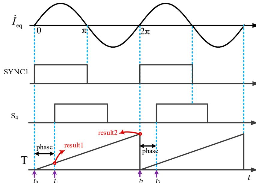
Figure 10. Principle of digital phase-locked loop.
